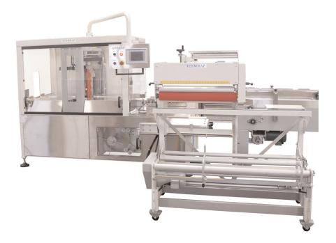
The 914 servo orbital vertical sealer is the machinery solution of choice for high speed endof-filling-line shrink packaging. Now products such as bottles, jars or cans are able to be wrapped while in the vertical position.
