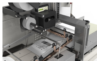
C. LABELER AND END SEAL The package stops on the exit conveyor of the wrapper where the proper bag size is sealed and the address label is automatically printed & applied.
