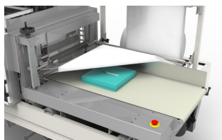
A. PRODUCT INFEEED AREA Random packages are accepted in the infeed area. As the packages arrive, the bar code is scanned and the address information is sent to the ID Technology print and apply labeler
