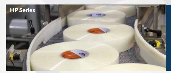
Ranging from 1.6 mil general purpose to 3.4 mil extremely tough options, HP Series hot melt packaging tapes combine an aggressive, high-tack adhesive with Hold Strong® technology to keep carton seals intact. HP Series packaging tapes are recommended for manual and automated industrial sealing of light to heavy weight cartons in a range of case sealing environments. Also available in specialty formulations for cold temperature environments and for sealing recycled cartons.
