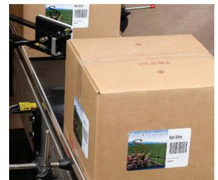
The systems also can be configured to label side and rear panels, or single panels. Use two Twin-Tamps for a 4-sided labeling solution.
